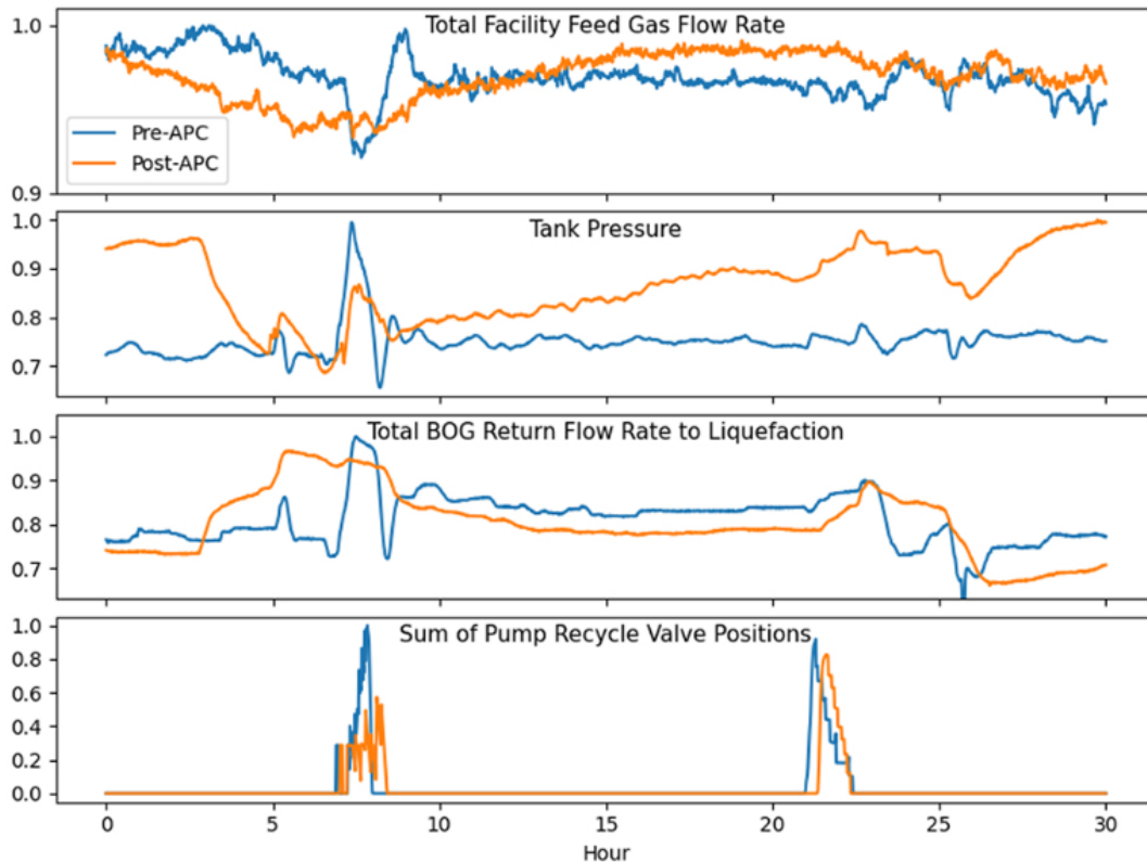
FIG. 4. Key process parameters during a shiploading event.
