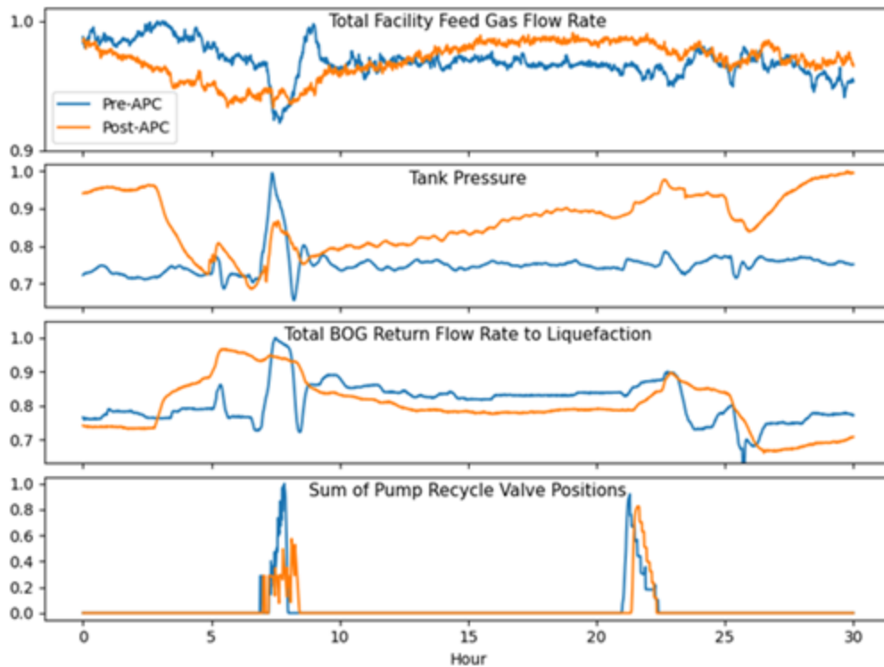
FIG. 4. Key process parameters during a shiploading event.
