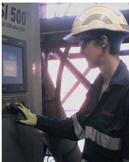
An operator uses the Outotec PSI 500 to check the size of iron ore particles at Rio Tinto's Paraburdoo mine.
